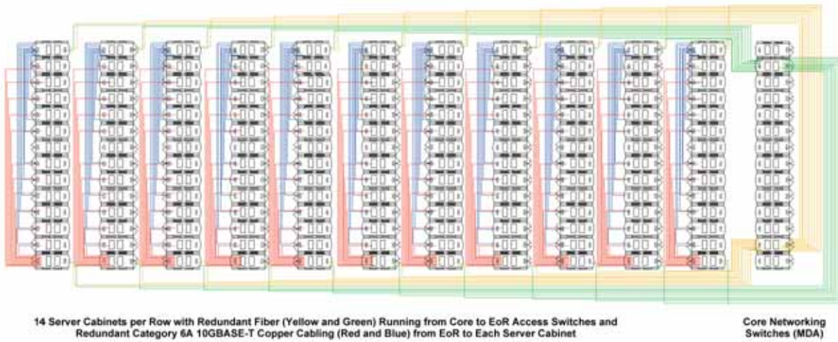
Figure 5: 144-Cabinet EoR Configuration
