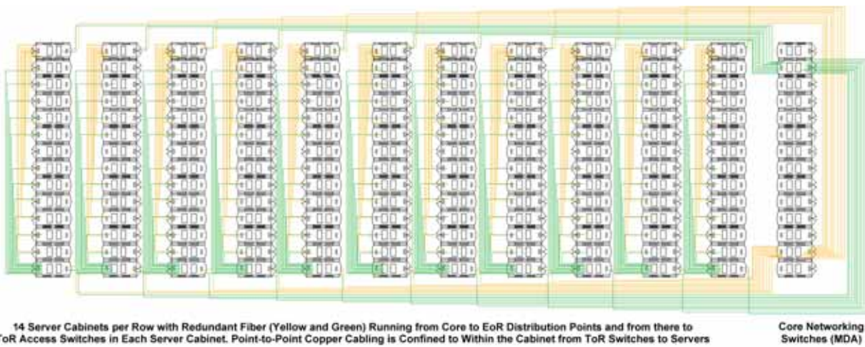
Figure 6: 144-Cabinet ToR Configuration
